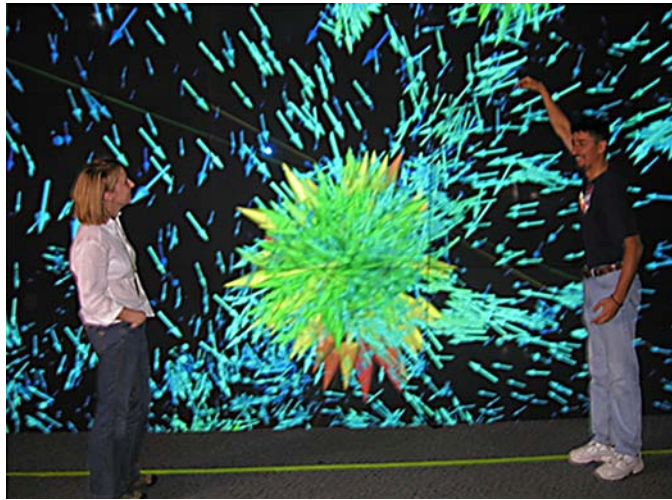
Figure 1. ParaView displaying a visualization of FLASH simulation data using vector arrow glyphs sized and colored by velocity magnitude on an 18 panel (3 by 6) tiled display wall.
